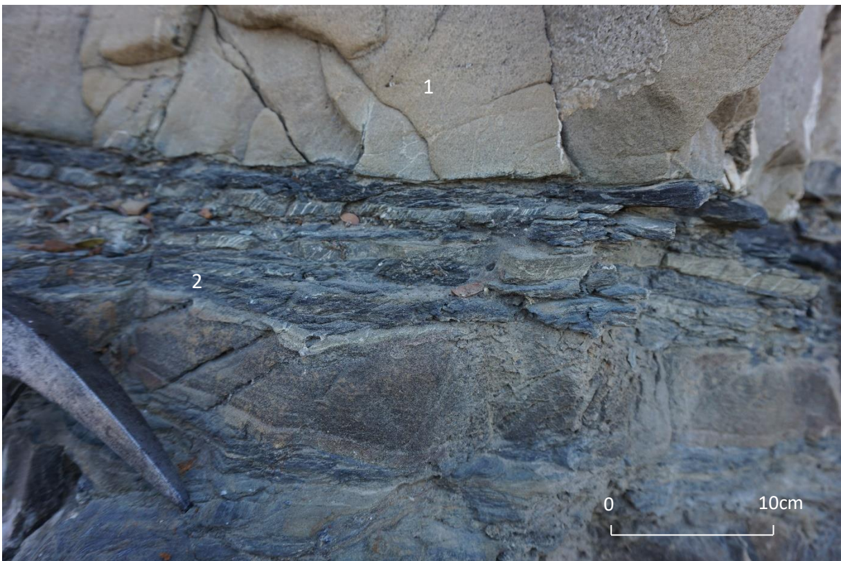
Thin shale beds between quartzite beds. 1: Quartzite, 2: There appears to be two cleavage planes within the shale.
