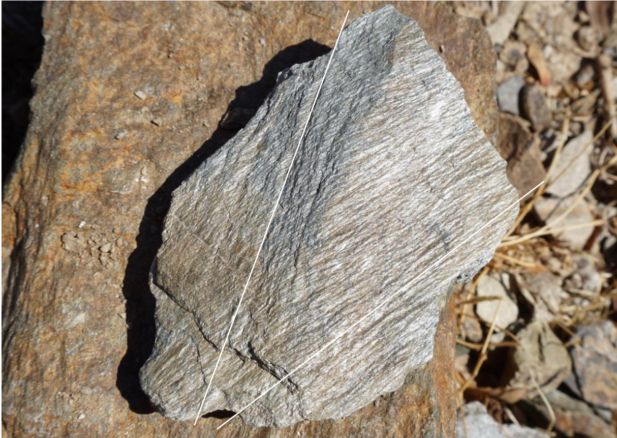
Phyllite hand sample showing two generations of cleavage ( S_1 and S_2 ).
