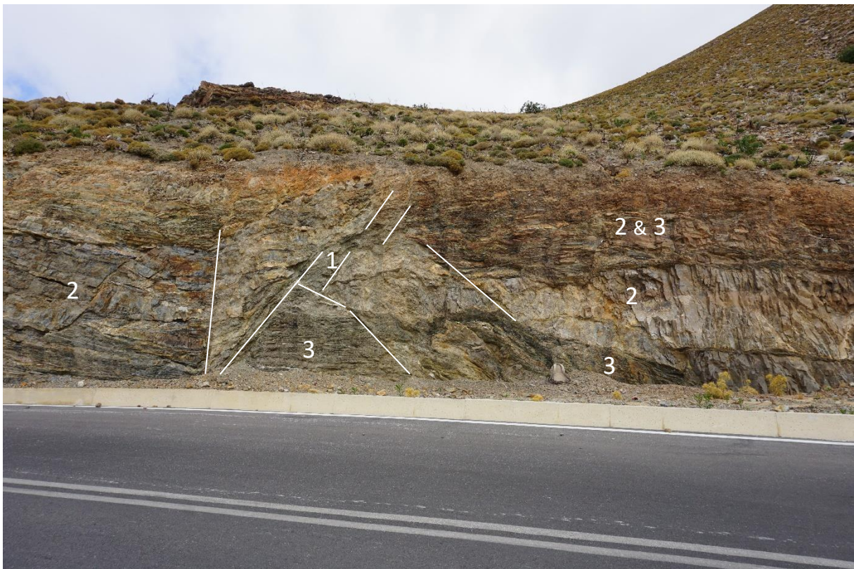
Overview of a Phyllite-Quartzite out-crop, displaying an array of faults. 1: Gauge zone, 2: Quartzite, 3: Phyllite
